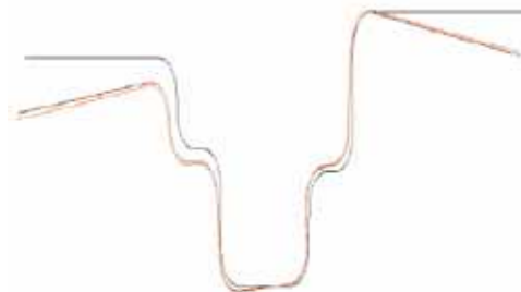
Figure 40. Calculation made by ESI on section C - AA5182 alloy
